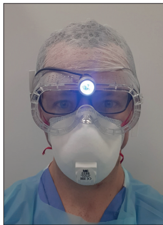
Figure 1: protective goggles with integrated LED headlight worn with full PPE
