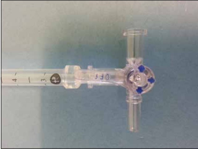
Fig 8. Three way tap attached to end of Manometer
